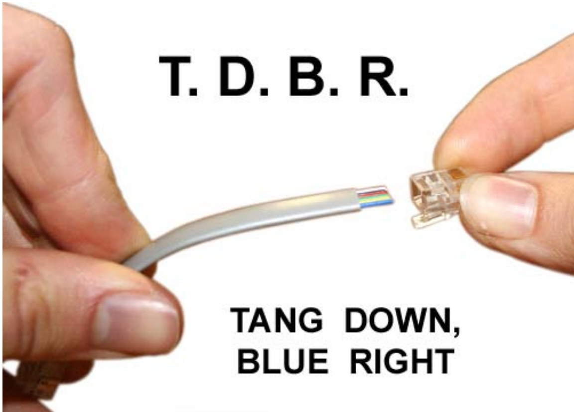
figure 09. Correct RJ Cable Orientation
