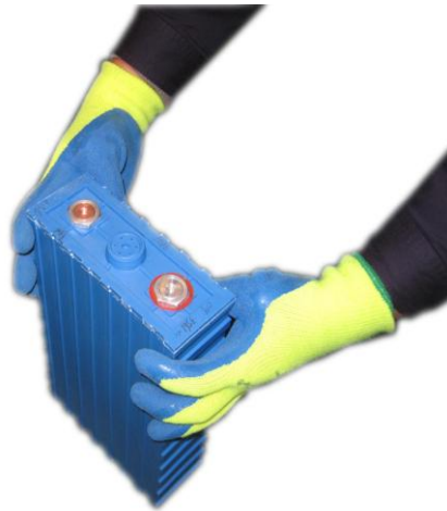
Picture 3.1.1.1: Keeping the battery pole upward
