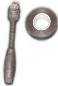
Picture 3.2.2.1: Tools need to be make strict insulated treatments
